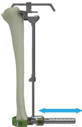
Once the correct height of the Cutting Block has been achieved, the Block may be pinned in place. It is recommended to use the most distal set of pin holes to allow the Cutting Block to be shifted further distally if necessary. The Angelwing may be passed through the cutting slot to check the saw blade trajectory prior to resection.
