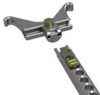
The Tibial Alignment Rod may then be assembled to the Monorail by depressing the side button and sliding the knuckle over the Monorail with the rod biased towards the Ankle Clamp.
