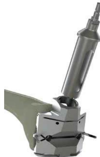
To remove the Halo Cutting Block from the femur, insert the Block Pusher into the halo on the Cutting Block and insert it as posteriorly as possible. Squeeze the grip of the Block Pusher to eject the Block from the femur. Alternatively, a mallet and small punch may be used against the edges of the Cutting Block to remove the block from the femur. Once the Cutting Block has been removed, the sides of the PS notch may be cleaned up with a saw blade to ensure the sides of the notch are parallel.
